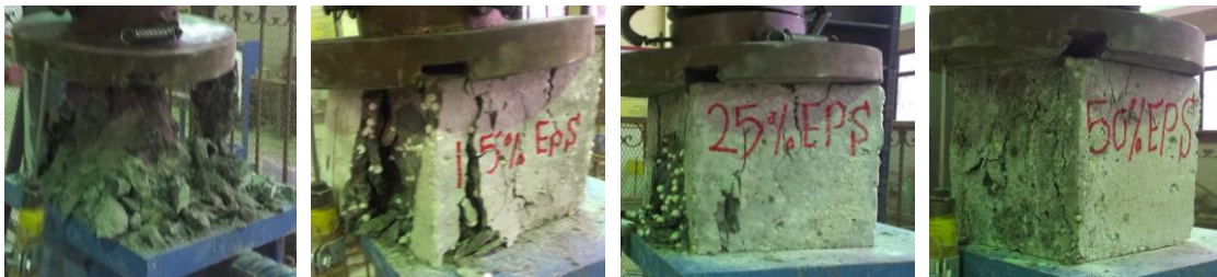
Fig. 2: Failure modes under compression of EPS foamed concrete different percentages specimens (0%, 15%, 25%, 35% and 50%).
