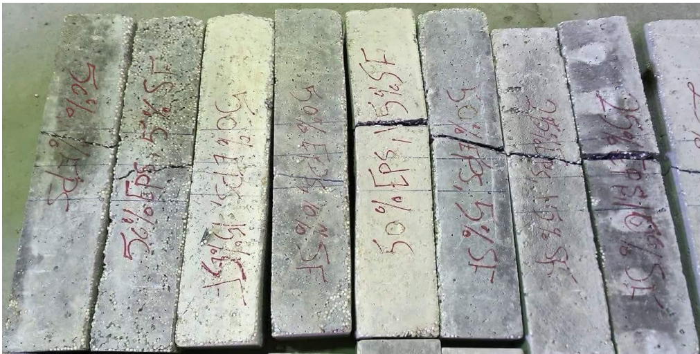
Photo 1: Failure modes of EPS foam concrete beams with SF percentages under flexural strength
