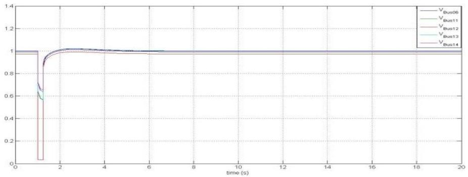
fig. 12. Voltages at nearing buses to bus 12 without PV penetration
