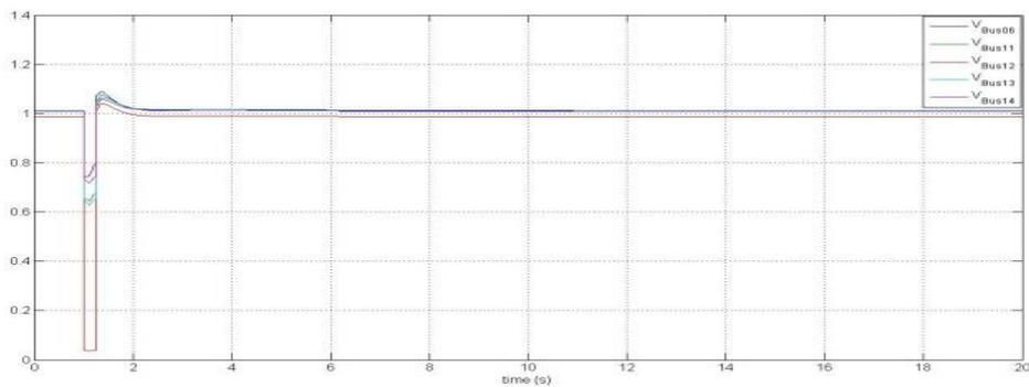
fig. 13. Voltages at nearing buses to bus 7 with 10% PV penetration
