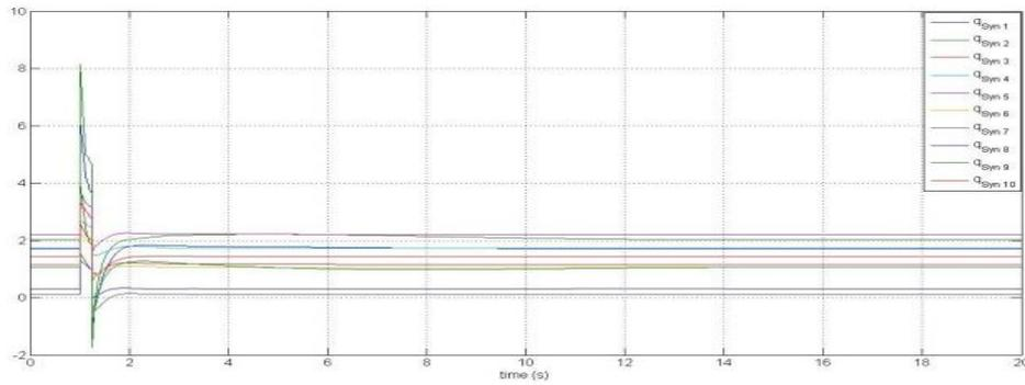
fig. 11. Reactive power of generators with 10% PV penetration
