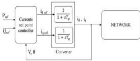
fig.2. PVGs Model 1 block diagram
