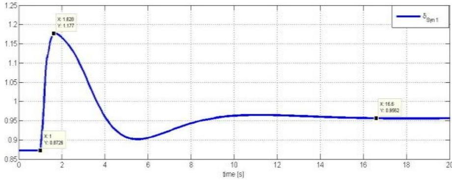
**fig. 6. Rotor angles of the slack generator without PV penetration**
