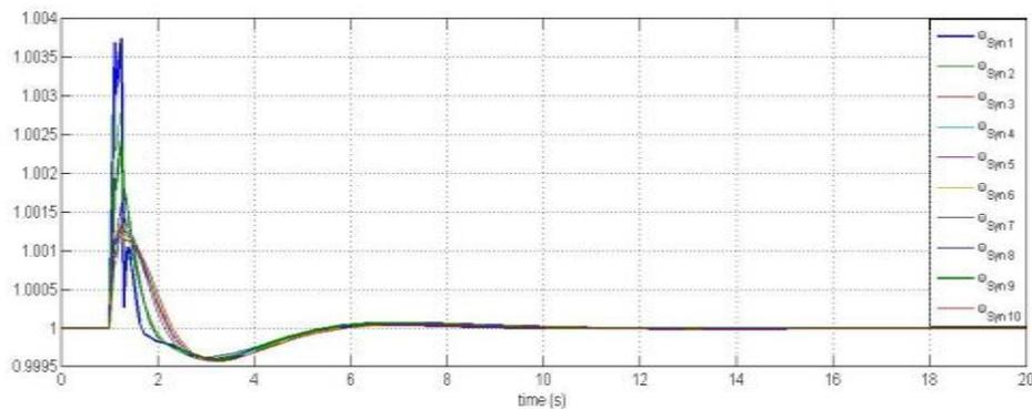
fig.14. Speeds of generators without PV penetration
