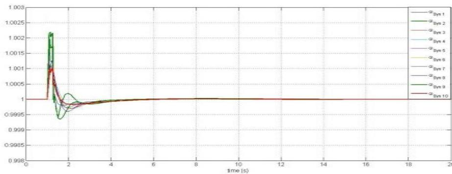
fig. 15. Speeds of generators with 10% PV penetration
