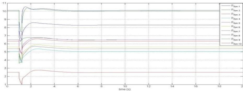
**fig.8. Active power of generators without PV penetration**
