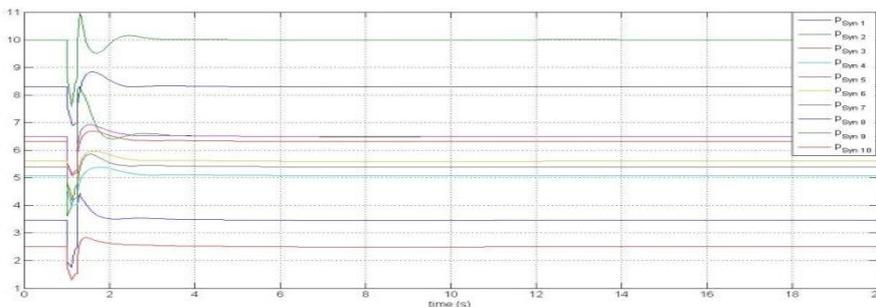
**fig. 9. Active power of generators with 10% PV penetration**
