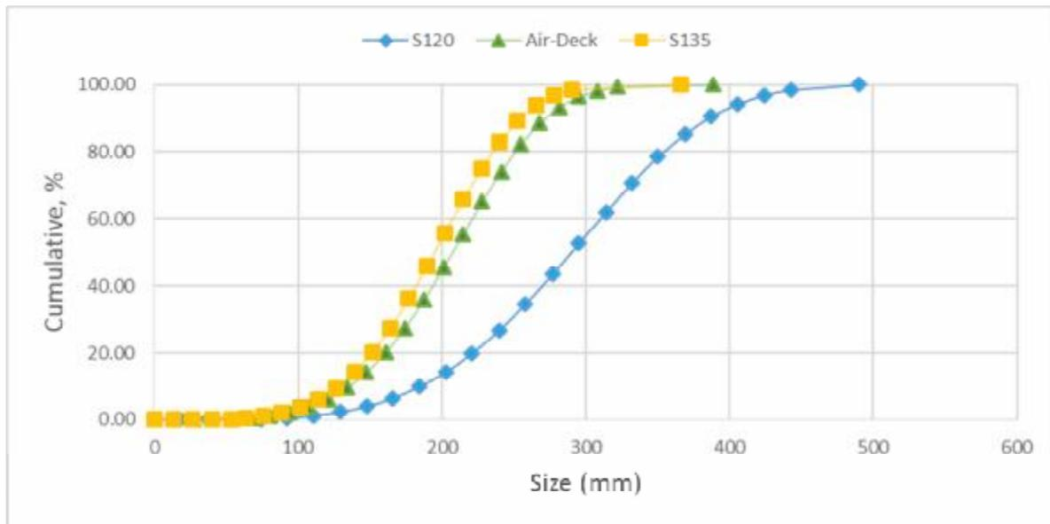
**Fig. 7. Blasting current state in comparing to using air deck and denser explosive**
