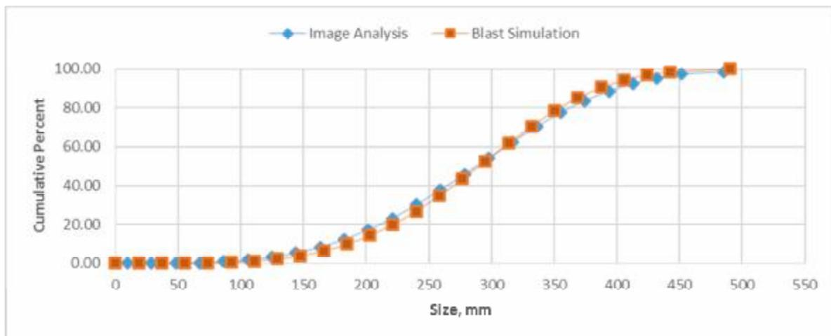
**Fig. 5. Fragmentations cumulative size distribution obtained from image analysis comparing to distribution obtained from blasting simulation**
