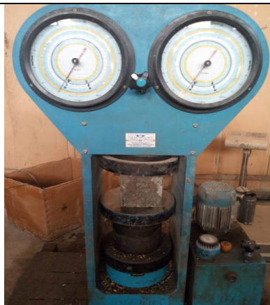
Fig.3. Machine of Test Specimens (Cubes and Cylindres and Prism).
