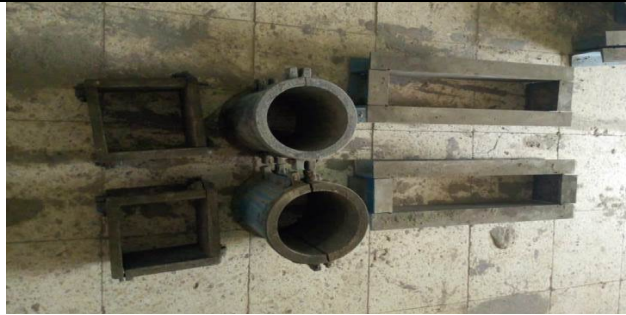
Fig.1. Cubes, cylinders and Prisms Molds.
