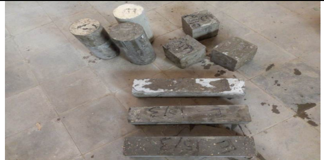
Fig.2. Concrete Specimens of Cubes, Cylinders and Prisms after Casting and Curing.
