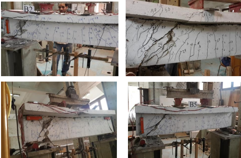
Fig 7: Failure mode for all beam specimens
