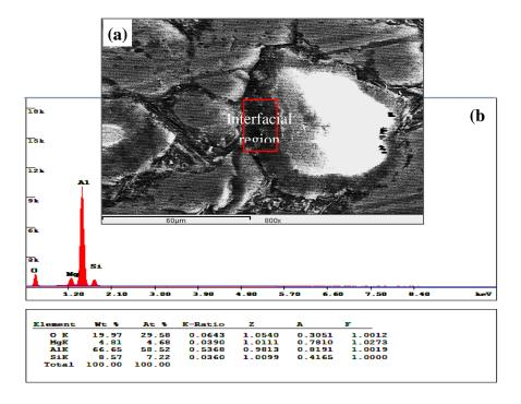
Fig.2: SEM/EDS analysis on the A356 alloy+ 20% Al<sub>2</sub>O<sub>3</sub>
