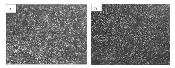
Fig.4: Optical micrographs of composites reinforced with A356 alloy+ 20%: (a) As cast, (b) Heat treated (100 X)
