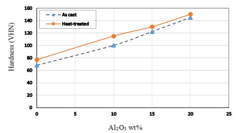
Fig.3: Effect of heat treatment on hardness of the test specimens
