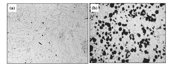
Fig.1: Optical micrographs of composites reinforced with: (a) A356 alloy, (b) A356 alloy+ 20% Al<sub>2</sub>O<sub>3</sub> (100 X)
