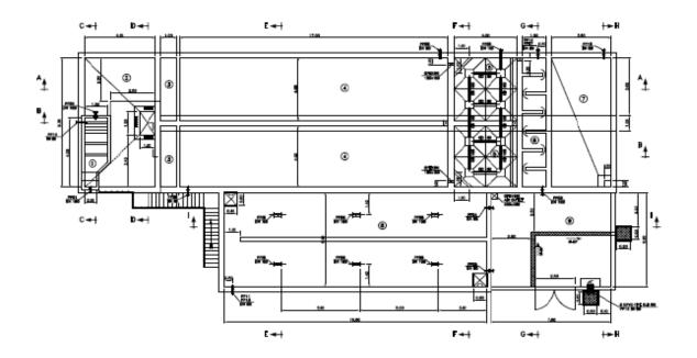
Figure 5. Plan of existing Extended Aeration W.W.T.P at red sea resort (executed by researcher).
