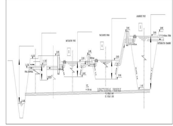
Figure 2. longitudinal cross-section in existing SPO W.W.T.P at Kafr ElShiekh Egypt
