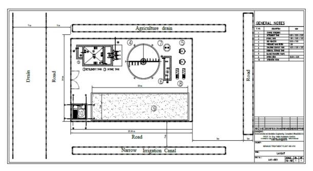
Figure 8. Layout of a D.H.S plant of 500m<sup>3</sup>/day at Egypt (Alex. Uni. service center).
