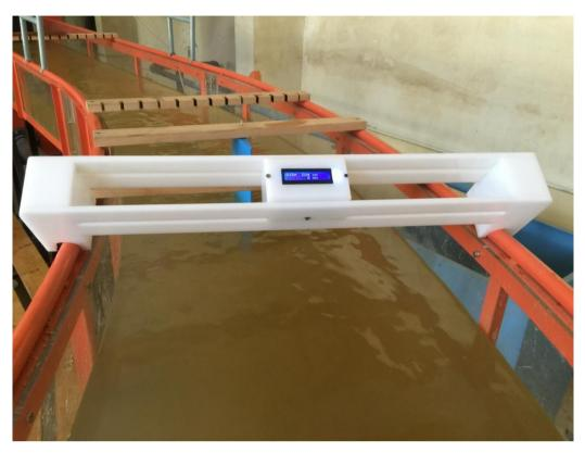
Photo: (2) Measuring device (Ultrasonic device - one spot).
