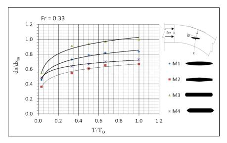
Figure: (11) The relation between  $(T/T_0)$  and  $(ds/ds_m)$  for all shapes
