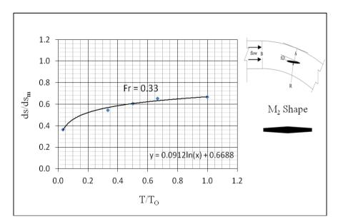
Figure (8): The relation between (T/TO) and (ds/dsm)
