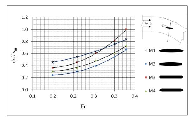
Figure: (6) The relation between (Fr) and (ds/ds<sub>m</sub>) for all shapes
