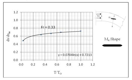
Figure: (10)The relation between (T/T<sub>0</sub>) and (ds/dsm)
