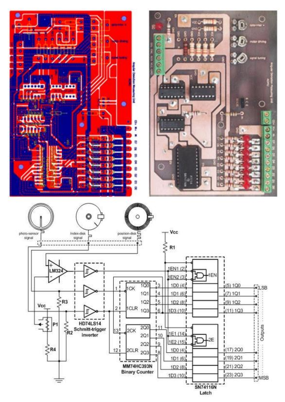
Fig (9) -Position determining circuit
