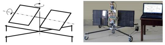
Fig (1) - A Dual-Axis Sun Tracker Over A Movable Structure
