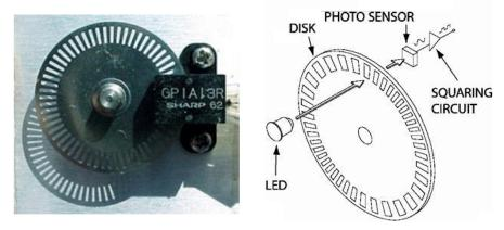
Fig (8) - Rotary-Disk Encoder
