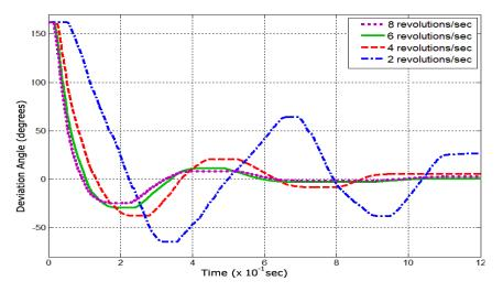
**Fig** (6) - **Delay Effect on process response**
