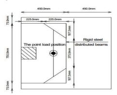
Fig.9: LVDT locations at bottom side
