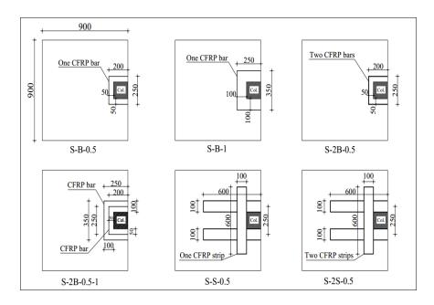
Fig.1: Strengthening schemes (All dimensions in mm)
