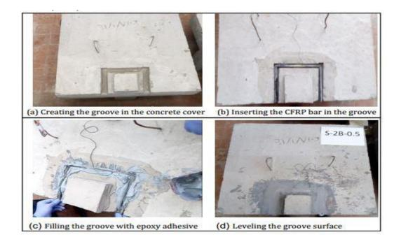
Fig.4: Strengthening procedures using NSM technique
