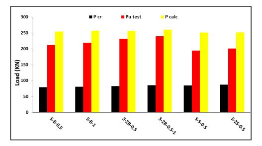
Fig. 15. Comparison between cracking load, experimental ultimate load and calculated ultimate load for the strengthened specimens
