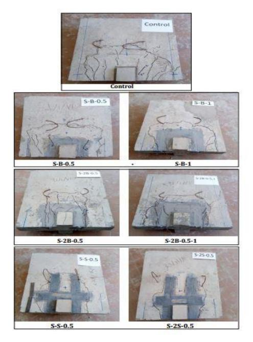
Fig.14: The tested specimens crack patterns at failure load (bottom faces)
