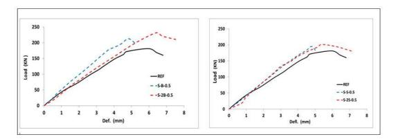
Fig.13: comparison of Load deflection based on the strengthening are
