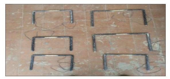
Fig. 3. CFRP bars used in this study
