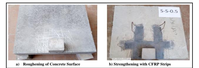
Fig.5: Strengthening procedures using EB technique
