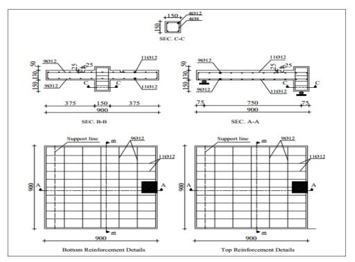
Fig.2: Dimensions and reinforcement details for specimens
