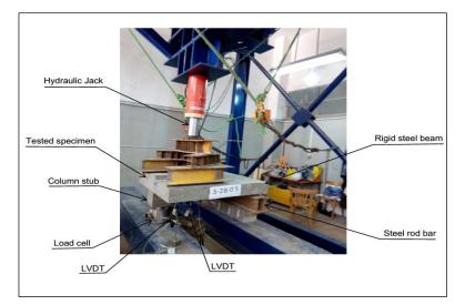
Fig.10. Set-up of Test
