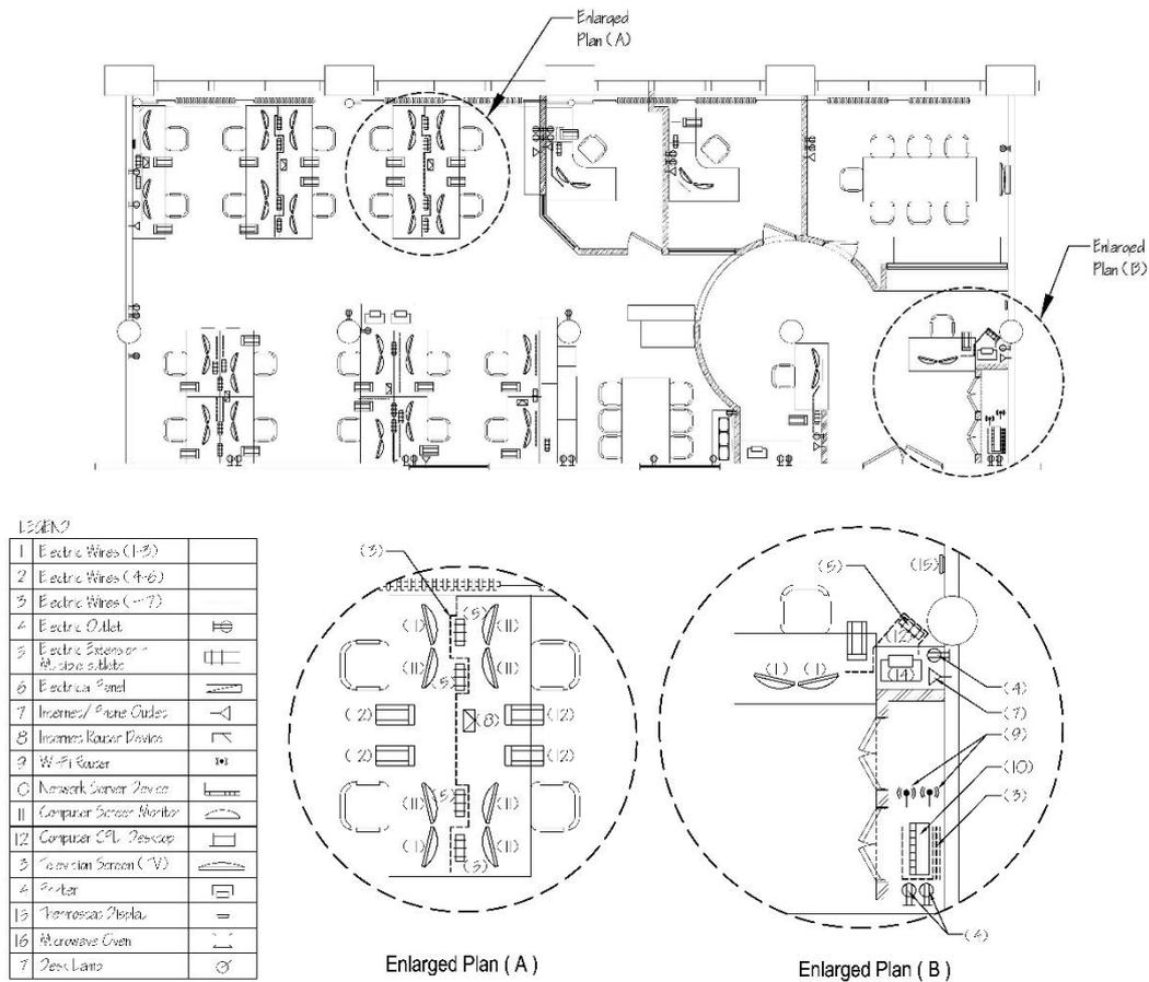
Figure 7: The space floor plan showing sources & devices emanating EMF/R.
