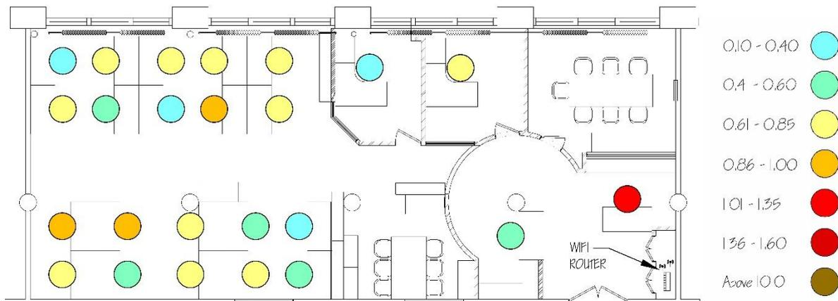
Figure 11: Average radio frequency measured at the chair of each working station.
