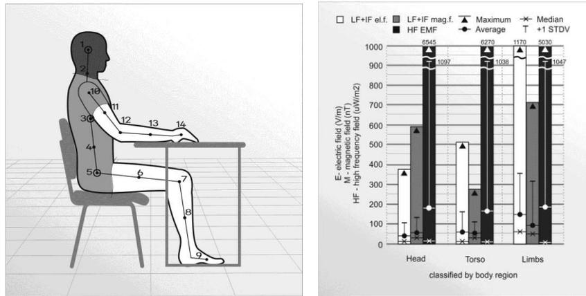
Figure 4. The 14-point measurement system by Koppel. Points are distributed into body regions as characterized by the vulnerability to the EMFs: head, torso, limbs.
