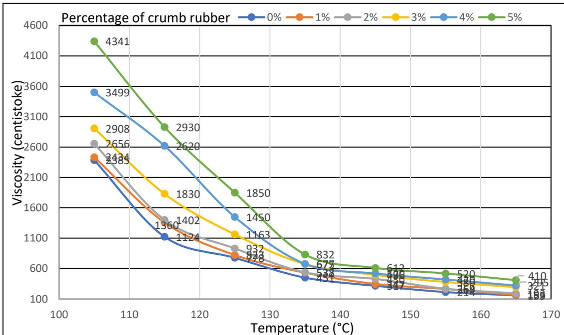
Fig 3: Relation between viscosity and temperature by adding crumb rubber
