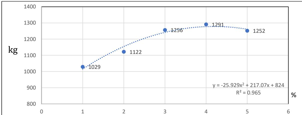
**Fig 4: Stability results for Crumb Rubber from recycled tires as additives**
