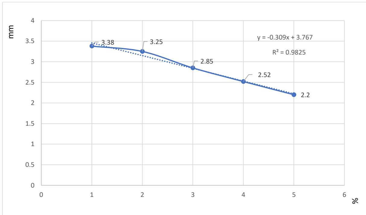
Fig 7 :Load wheel track rutting test results for Crumb Rubber from recycled tires.
