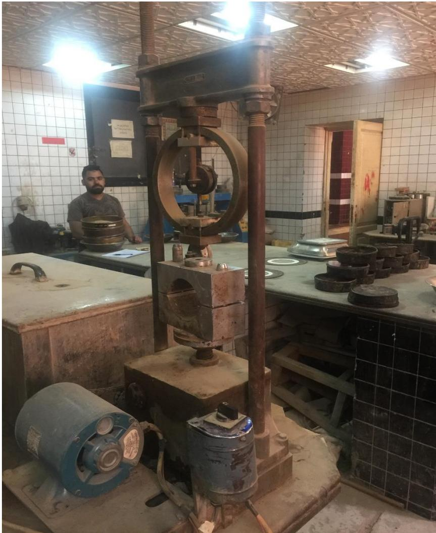
**Fig 2: Marshal stability- flow test**
