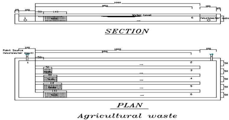
**Figure (1) Plan and Section of the Applied Pilot**
