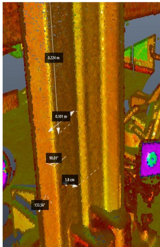
Fig 4. Using Recap Point Cloud programs to measure imperfection of specimens
