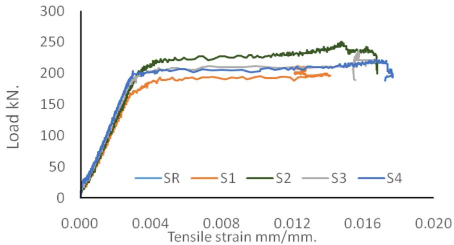
**Fig. 9:** The Relation between Load and Maximum Tensile Strain for Tested Beams
