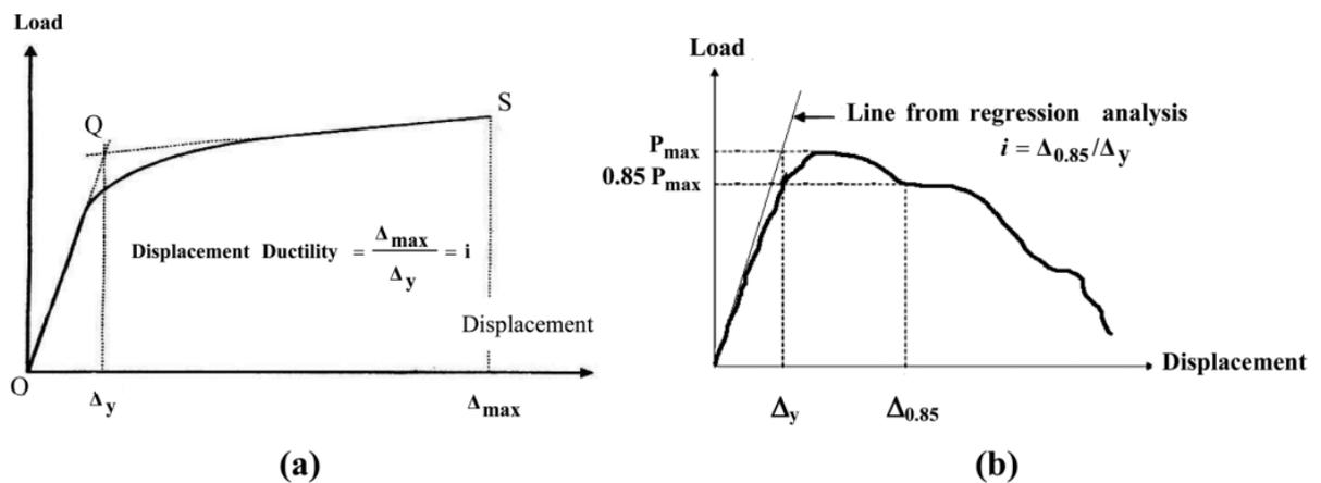
**Fig.13:** Definition of Displacement-Ductility Ratio
