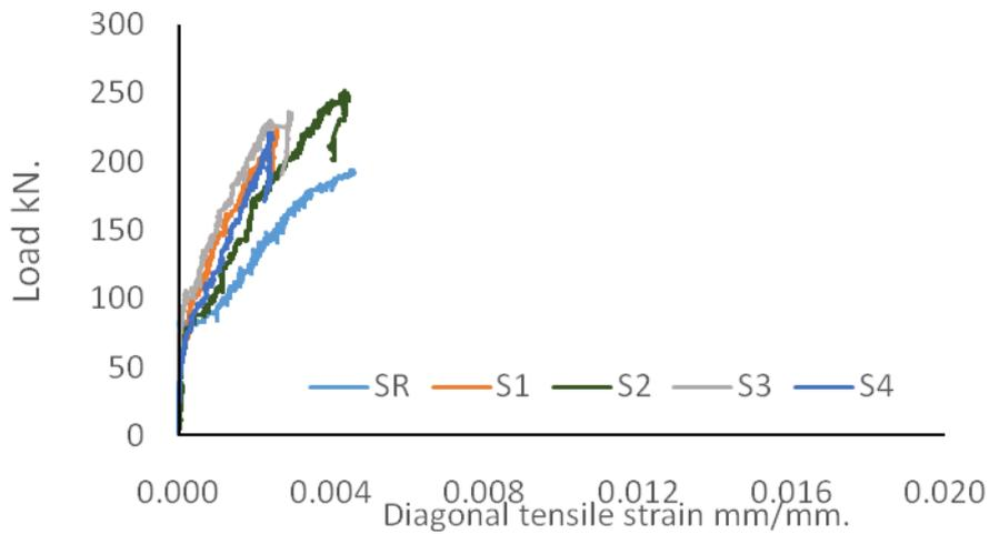
**Fig. 10:** The Relation Between Load and Maximum Diagonal Tensile Strain for Tested Beams
