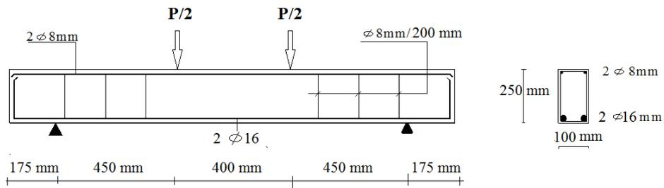
**Fig .3:**The Beam Dimensions and Reinforcement Details of the Beam Specimens
