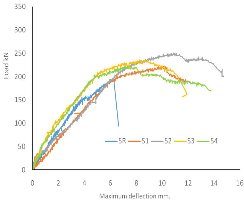
**Fig.8:** The Relation between Load and Maximum Deflection for Tested Beams
