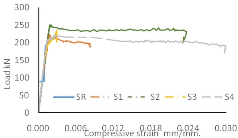
**Fig. 11:** The Relation between Load and Maximum Compressive Strain for Tested Beams
