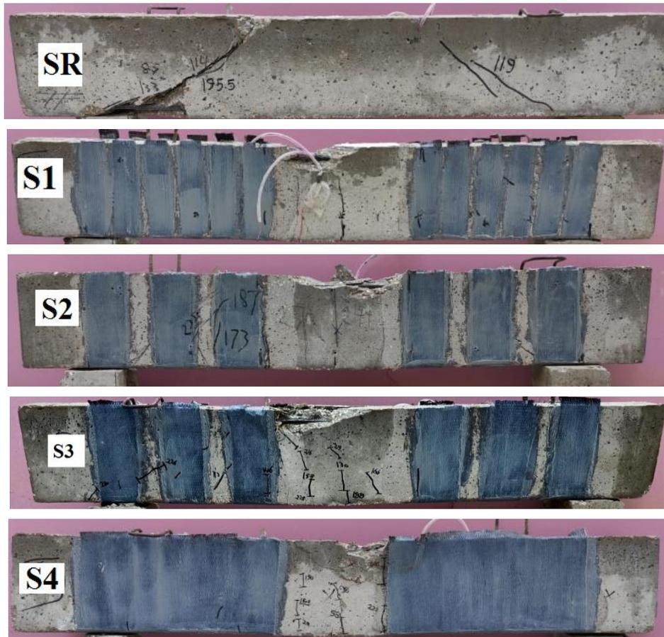
**Fig. 12:** Cracking Patterns and Modes of Failure at Ultimate Load for Tested Beams
