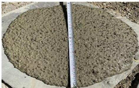
**Fig.1:** The Slump Flow Diameter for SCC mixture
