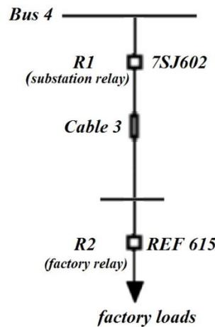
**Fig. 2:** Feeder components with its protective elements
