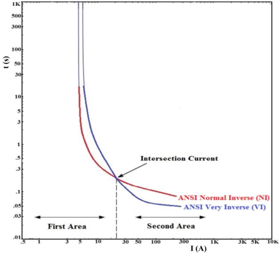
Fig. 3: The used relay curve types
