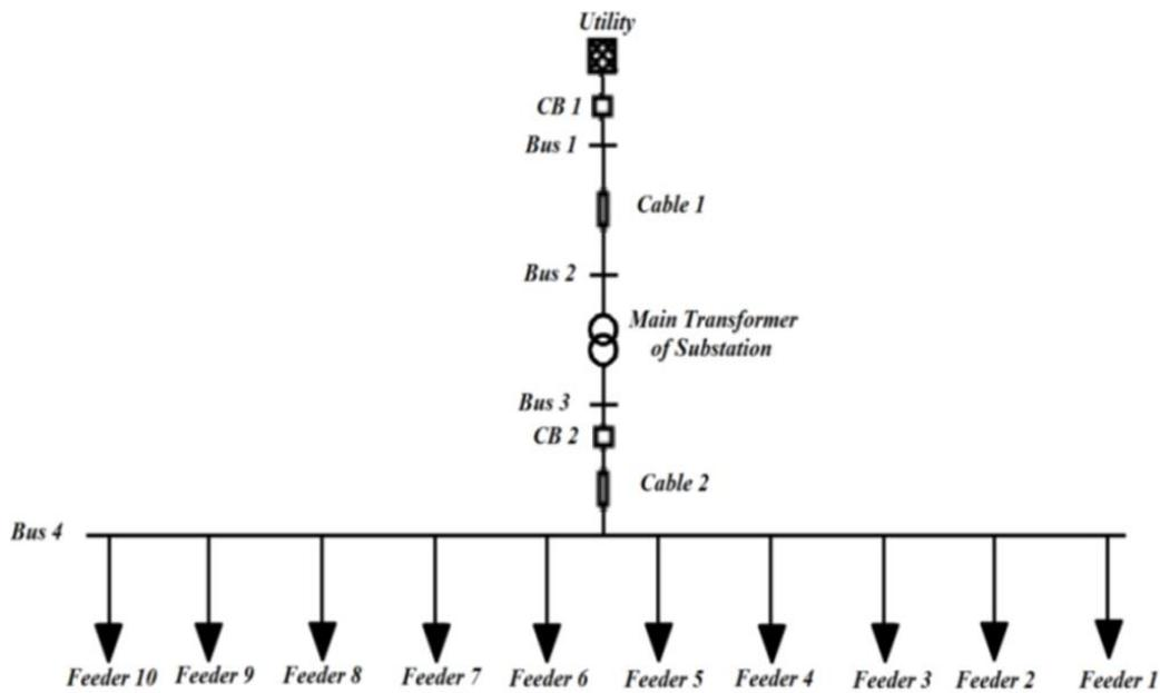
**Fig. 1:** Single Line Diagram of real radial system
