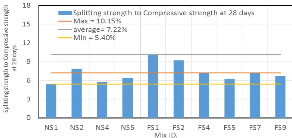
**Fig. 9: The ratio between splitting strength to Compressive strength (SCR) at 28 days.**
