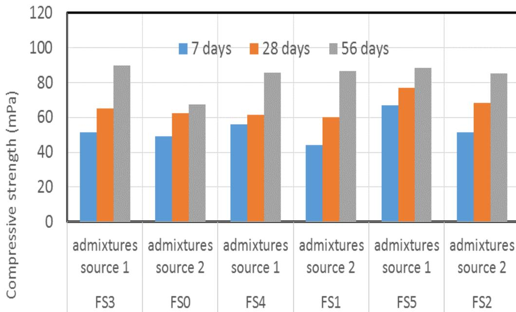
**Fig. 7: The effect of admixtures source on compressive strength**
