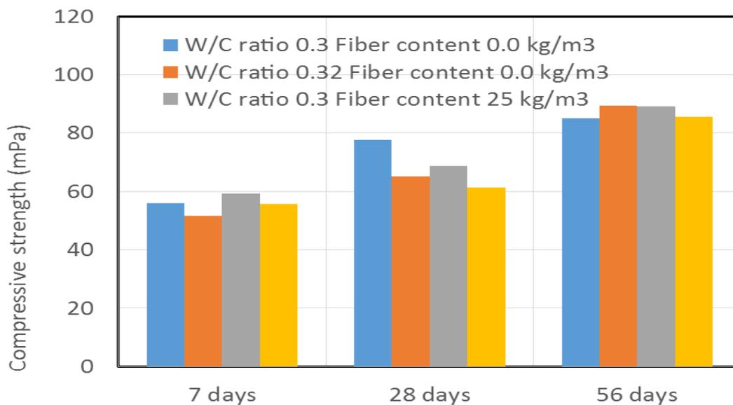
**Fig. 8: The effect of W/C ratio on compressive strength.**
