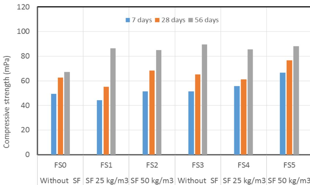
**Fig. 5: The compressive strength for mixes FS0 to FS5**
