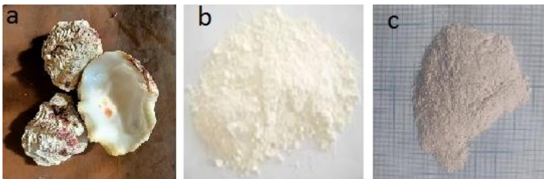
Fig 1: (a) Oyster shell collected from red sea (b) oyster shell powder after crushing in ball mill (c) Oyster shell powder after calcination for 1000 °C for a period of 1 hour
