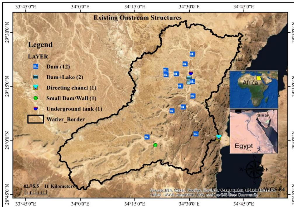
**Fig. 2:** layout and the existing structures in Wadi Watier Basin.
