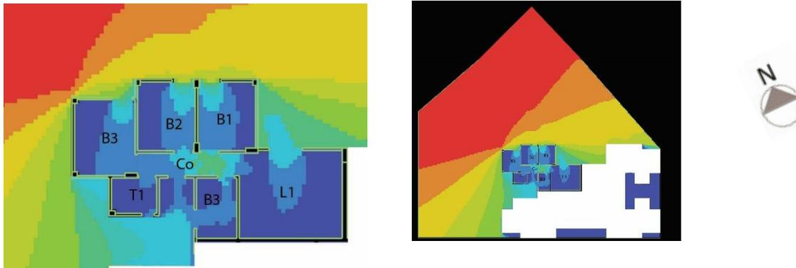
**Figure 10:** The VGA map of the connectivity value relative to the floor plan (the arrow represents the wind direction; from red to deep blue, the connectivity is from big to small) source: Author.
