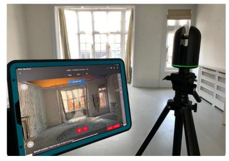
Figure 4: LeicaBLK laser scanner.
