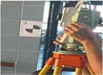
Figure 2: Example of targets used in fieldwork.
