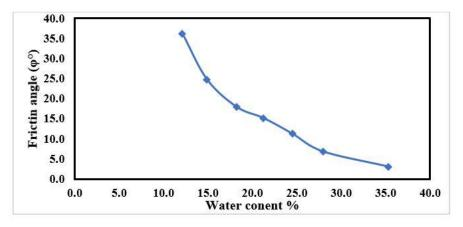
Fig. 5: relation between the friction angle & the water content %
