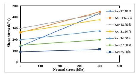
Fig. 4: Relation between shear stress and normal stress at water content from 12.20% to 35.00%
