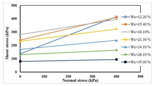
Fig. 1: Shear stress and normal stress relationships at water contents from 12.2% to 35%
