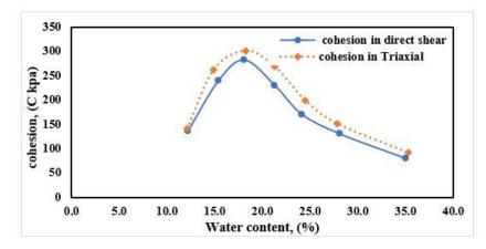
Fig. 7: Comparison between the Cohesion in direct shear and triaxial test at water content from 12.2% to 35%.
