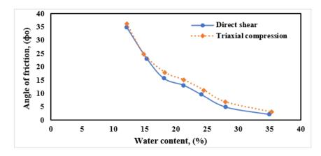
Fig. 8: Comparison between the friction angle in shear and triaxial test at water content from 12.2% to 35%.
