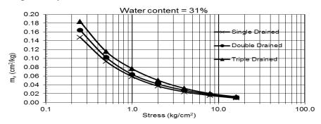
Fig. 4: Relationship between the coefficient of volume change (m<sub>v</sub>) and stresses for different drainage at water content 31%
