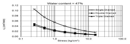
Fig. 11: Relationship between coefficient of consolidation (c<sub>v</sub>) and stresses for different drainage at water content 47%
