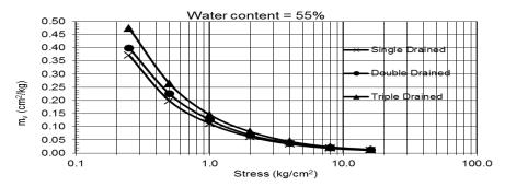
Fig. 7: Relationship between the coefficient of volume change (m<sub>v</sub>) and stresses for different drainage at water content 55%
