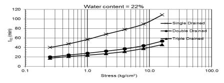
Fig. 13: Relationship between time of consolidation (t<sub>50</sub>) and stresses for different drainage at water content 22%
