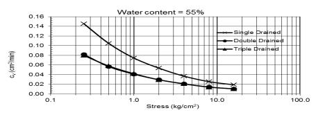
Fig. 12: Relationship between coefficient of consolidation (c<sub>v</sub>) and stresses for different drainage at water content 55%
