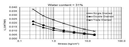
Fig. 9: Relationship between coefficient of consolidation (c<sub>v</sub>) and stresses for different drainage at water content 31%
