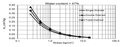
Fig. 6: Relationship between the coefficient of volume change  $(m_v)$  and stresses for different drainage at water content 47%
