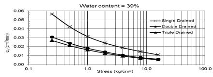
Fig. 10: Relationship between coefficient of consolidation (cv) and stresses for different drainage at water content 39%
