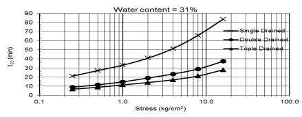
Fig. 14: Relationship between time of consolidation (T<sub>50</sub>) and stresses for different drainage at water content 31%
