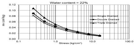
Fig. 3: Relationship between the coefficient of volume change  $(m_v)$  and stresses for different drainage at water content 22%
