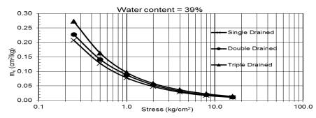
Fig. 5: Relationship between the coefficient of volume change (m<sub>v</sub>) and stress for different drainage at water content 39%
