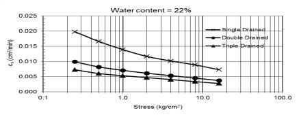
Fig. 8: Relationship between coefficient of consolidation (cv) and stresses for different drainage at water content 22%
