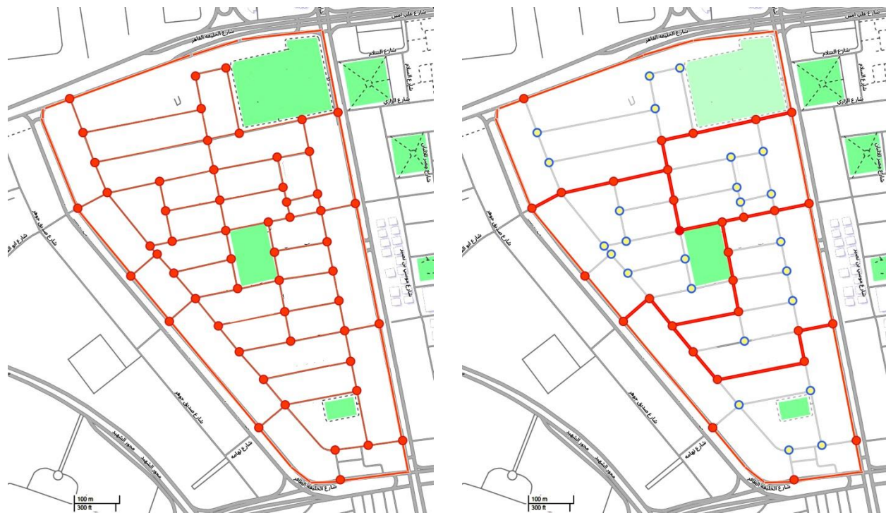
Fig. 9: Left: Map showing the region nodes currently. Right: Map showing the region after applying superblock strategy. Edited by Researcher
