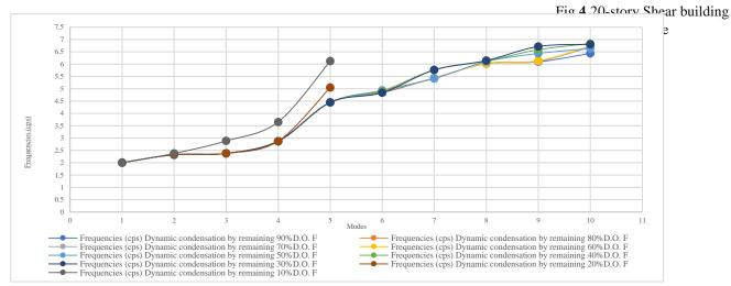
selecting the master degrees of freedom accurately once (keep the DOFs in which displacements are Fig. 5 Comparison of frequencies when removing different numbers of degrees of freedom 10%, 20%, 30%, 40%, 50%, 60%, 70%, 80% and 90%, respectively
