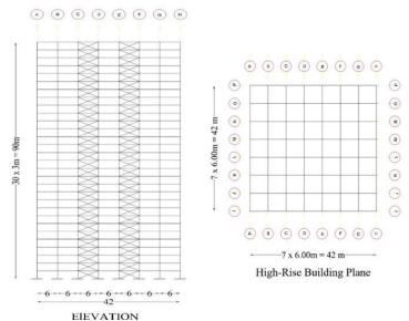
Fig.9 A 30-storey steel frame building (42x42) with Hight= 30x3.0= 90.m.
