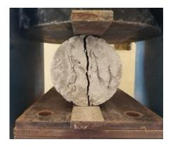
Fig. 5. Indirect tension test.
