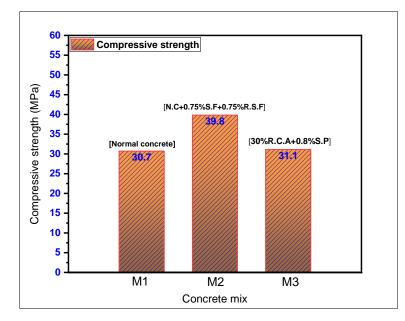
Fig. 7. Compressive strength for three different concrete mixes after 28 days.
