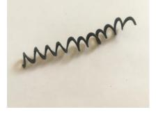
Fig. 2. Corrugated segment industrial steel fiber shape.
