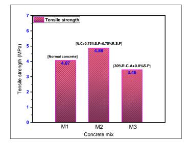
Fig. 8. Tensile strength for three different concrete mixes after 28 days.
