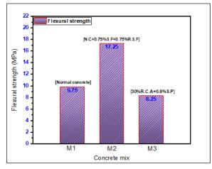
Fig. 9. Flexural strength for three different concrete mixes after 28 days.
