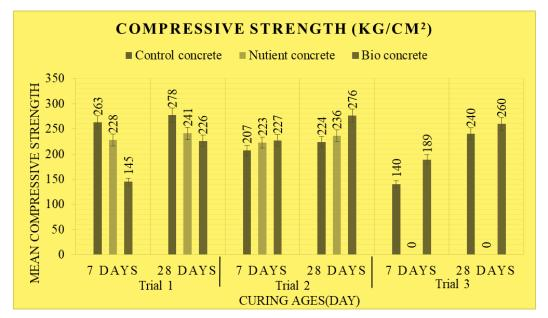
Fig. 10. Charts the compressive strength test results for hardened concrete in three trial
