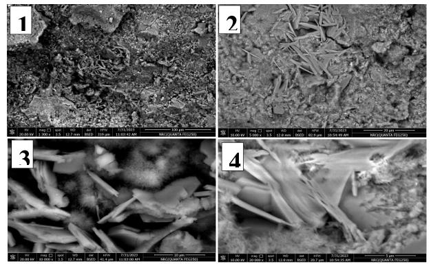
Fig. 15. Scanning electron micrographs of bio-concrete and control specimens (1 at 1300), (2at 5000), (3 at 10000) and (4 at 20000X).
