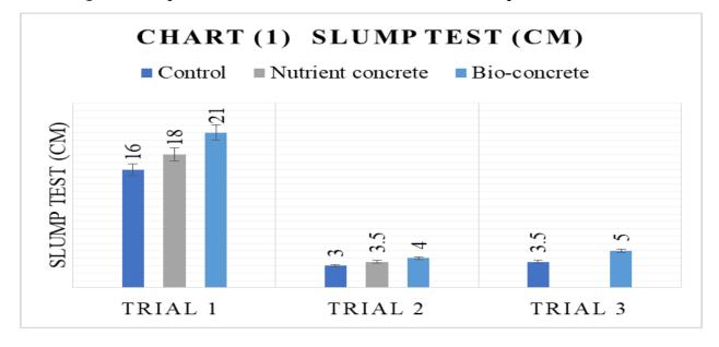
Fig. 9. Charts the slump test results for fresh concrete in three trial mix.
