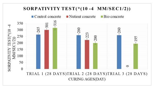
Fig. 13. Charts the sorpativity test results for hardened concrete in three trial mix.
