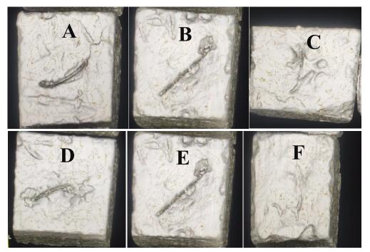
**Fig. 14.** X rays CT test for Concrete sample from 2 trial mix where: (A and D) Control concrete, (B and E) Nutient concrete and (C and F) Bio concrete.
