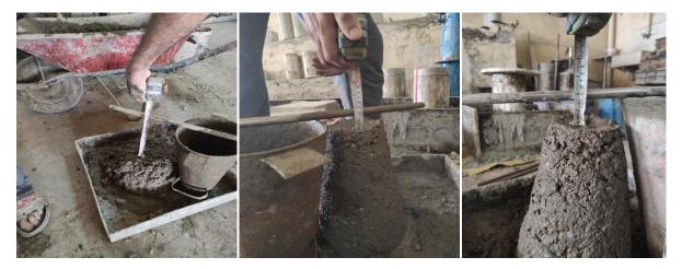
Fig. 8. Some pictures of three mixtures for concrete Slump of fresh concrete.
