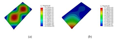
**Fig. 7.** Deformed Profile of the Slab used in Case Study-C60 (a) Before Column Removal and (b) After Column Removal.
