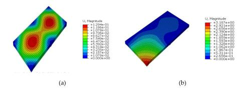
**Fig. 10.** Deformed Profile of Slab having Thickness of 160mm (Case Study-C160) (a) Before Column Removal and (b) After Column Removal.
