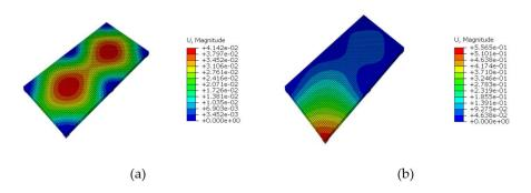
**Fig. 8.** Deformed Profile of the Slab used in Case Study-C80 (a) Before Column Removal and (b) After Column Removal.
