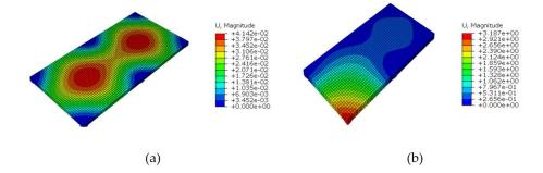
**Fig. 9.** Deformed Profile of Slab having Thickness of 125mm (Case Study-C125) (a) Before Column Removal and (b) After Column Removal.
