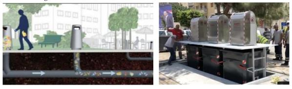
Fig. 3. Collection through Underground Waste Collection System [13].
