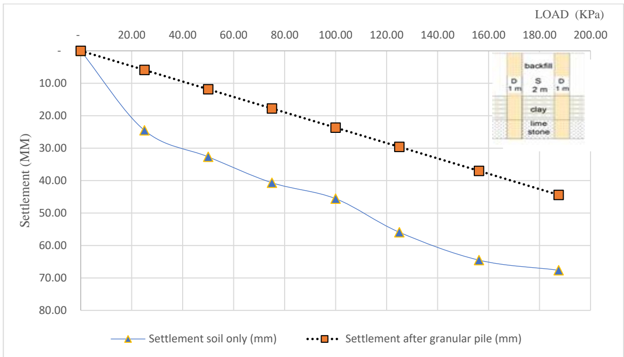
Fig.13. Stresses & Settlement relationship for soil from Analytical calculation before and after construction of granular pile.
