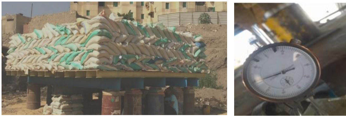
Fig.9. Details about the loading devices and sample of readings of the dial gauge .
