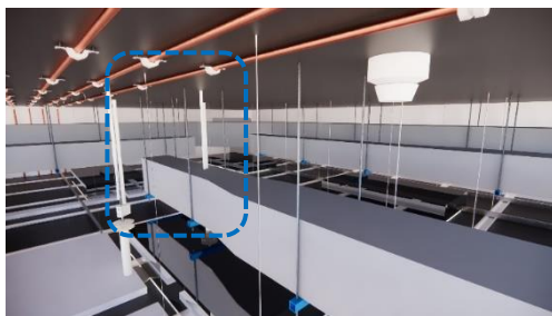
a. Medical instrument fixations conflict with ceiling lighting fixtures and with HVAC duct.
