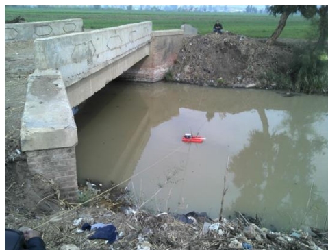
Figure 1: Velocities and bathymetry measurements at the six cross sections using ADCP device.
