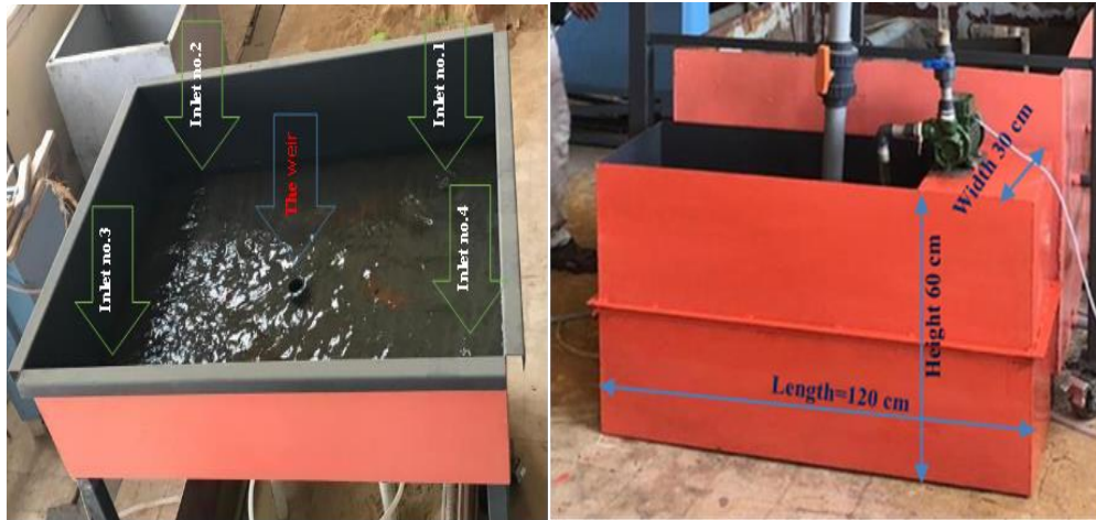
Photo. 5. Source Tank and Upper Tank.
