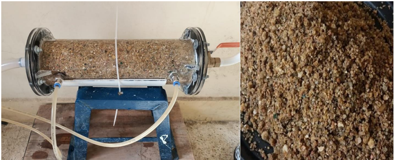
Figure (6). Sandy Gravel Soil Sample.
