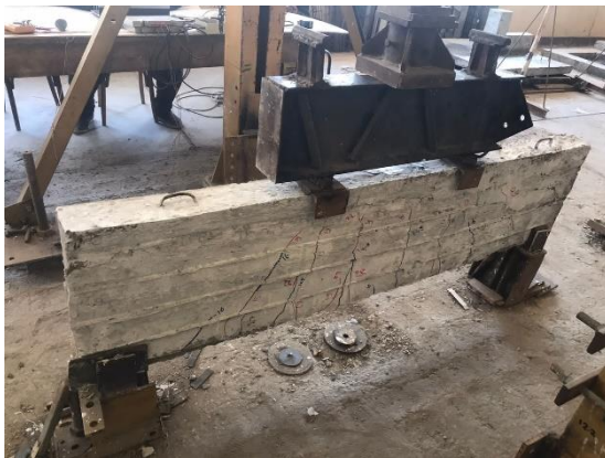
Figure 13 : Crack on the beam (15-350) ( Experimental )
