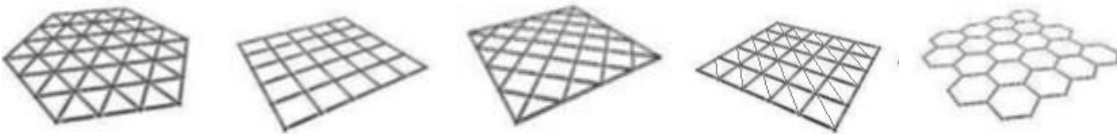
Fig. 2. Basic patterns for grid geometry.
