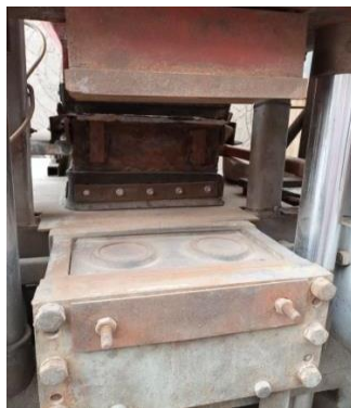
(b) Mould form lower face
