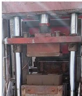
(e) The Compacted Unit –Raised
