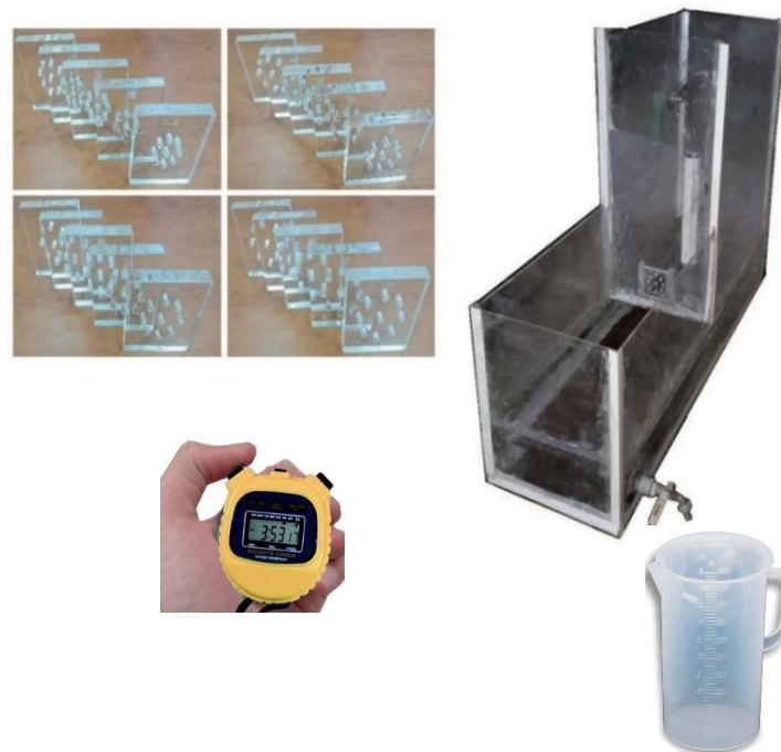
Fig. 2: Real photo of the physical model and orifice plates
