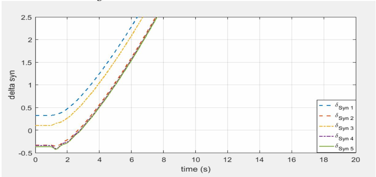
Fig.21. Represent Delta Against Time For All Generators When The Line 2-4 Outage From The Network Without Control
