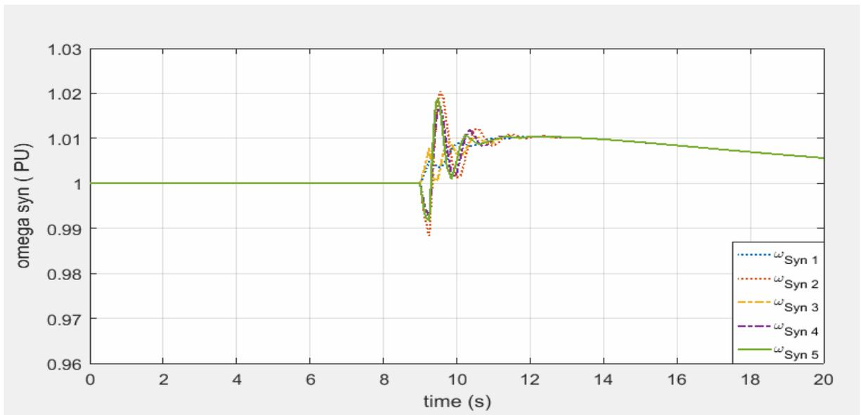
**Fig.17. Represent speed against Time for All Generators When the Fault Occurs At Bus No.2 – Without Control**
