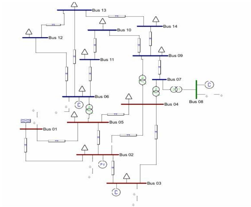
**Fig. 11. Show the single line diagram for 14 Bus Network**
