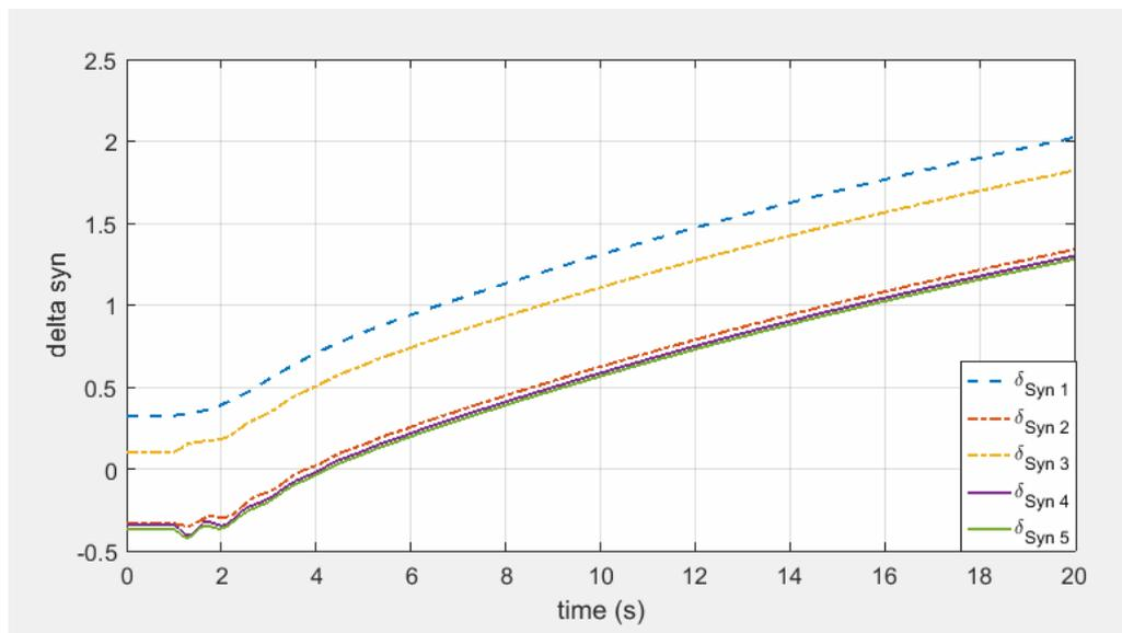
**Fig.23. Represent delta against Time for All Generators When the line 2-4 outage from the network with control.**
