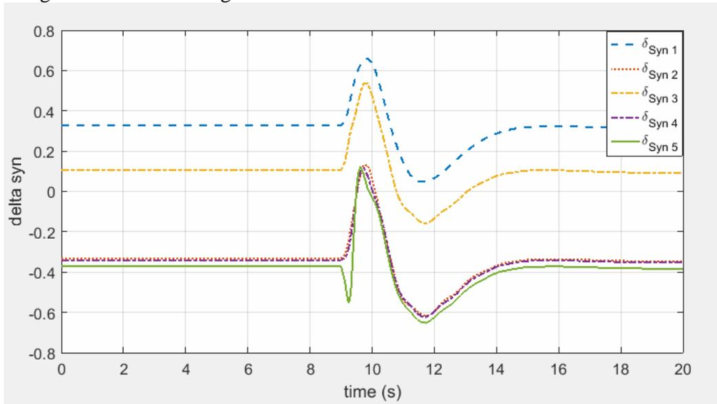
**Fig. 14. Represent delta against Time for All Generators When the Fault Occurs At Bus No.11 – With AVR, TG and PSS Control are used**
