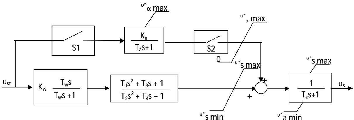
Fig. 8. Power system stabilizer Type V
