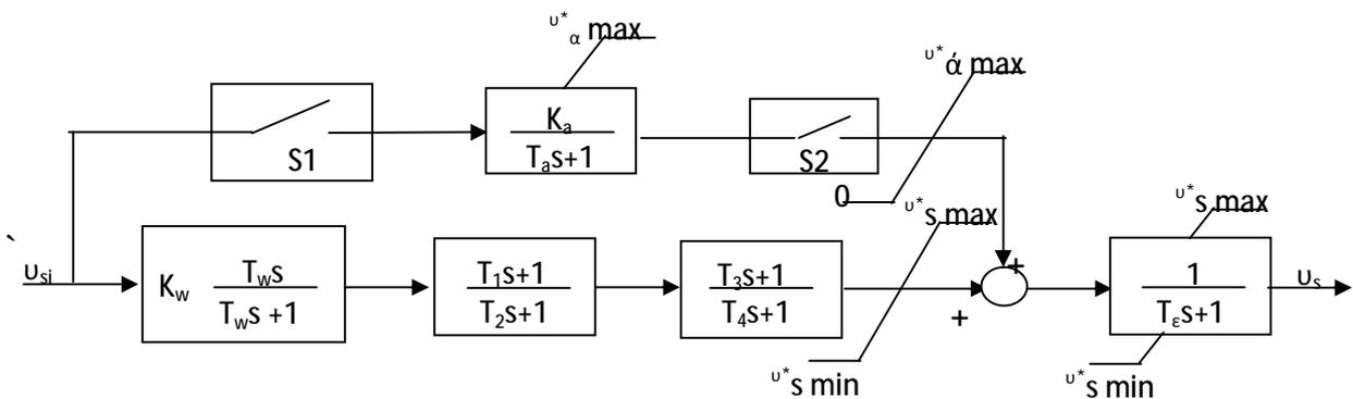
Fig.7. Power system stabilizer Type IV.
