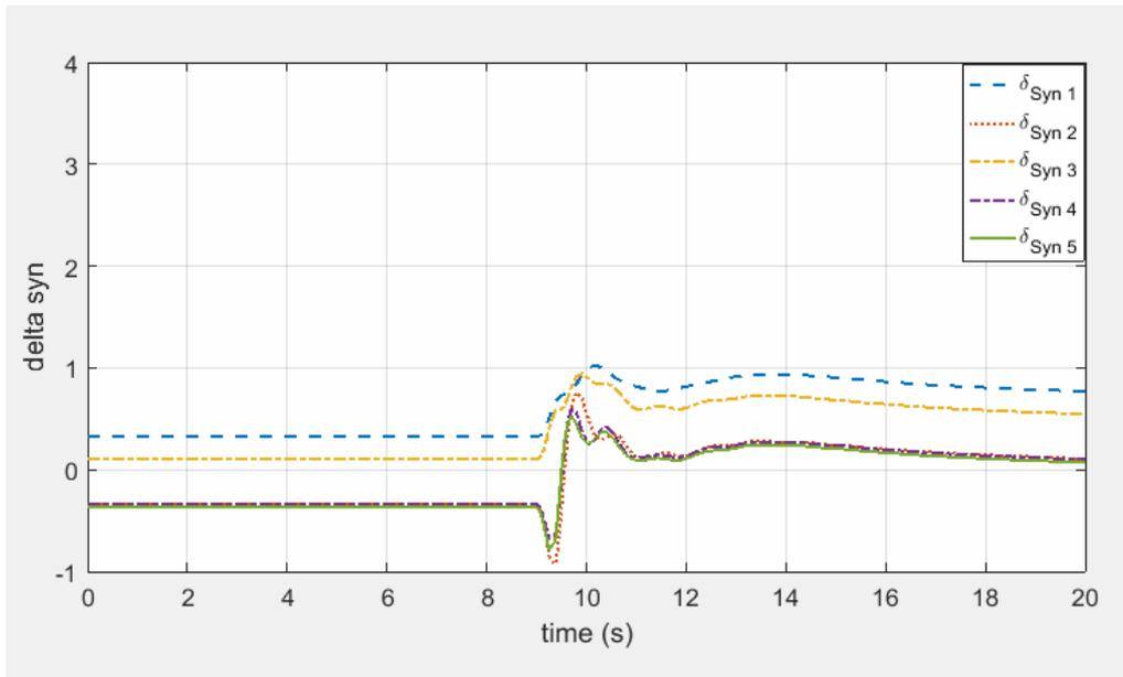
**Fig.18. Represent delta against Time for All Generators When the Fault Occurs At Bus No.2 – With AVR, TG and PSS Control**
