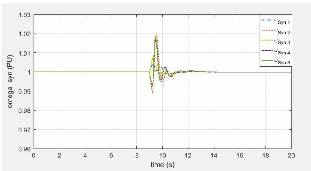
**fig.19. Represent speed against Time For All Generators When The Fault Occurs At Bus No.2 – With AVR, TG and PSS Control**
