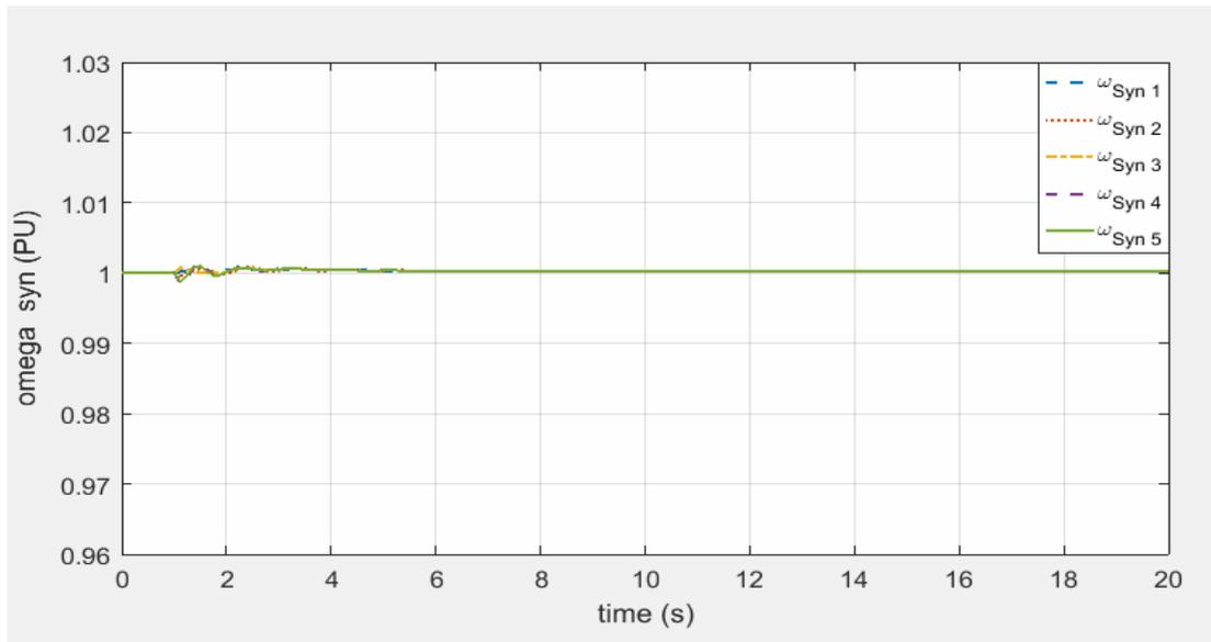
Fig.24. Represent speed against Time for All Generators When the line 2-4 outage from the network with control.
