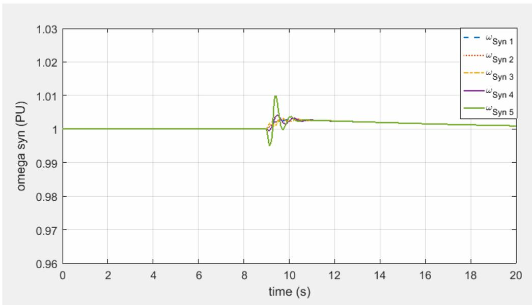
**Fig. 15. Represent speed against Time for All Generators When the Fault Occurs At Bus No.3 – With AVR, TG and PSS Control are used**
