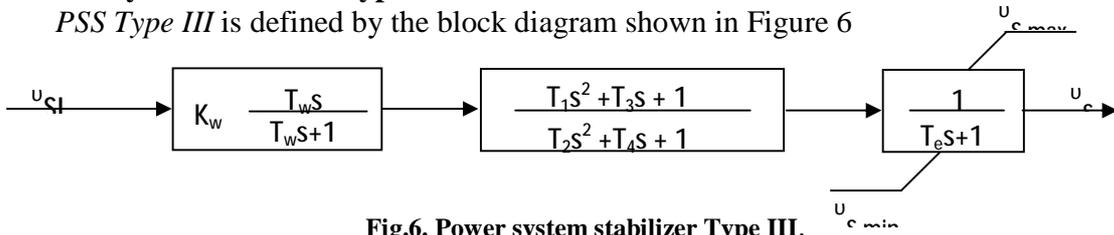
Fig.6. Power system stabilizer Type III.
