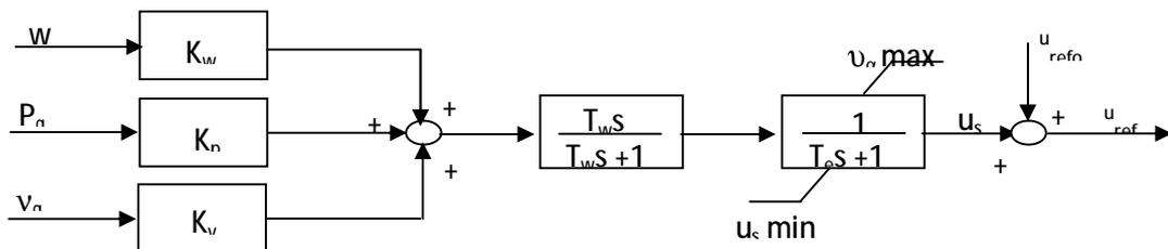
Fig. 4. Power system stabilizer Type I.
