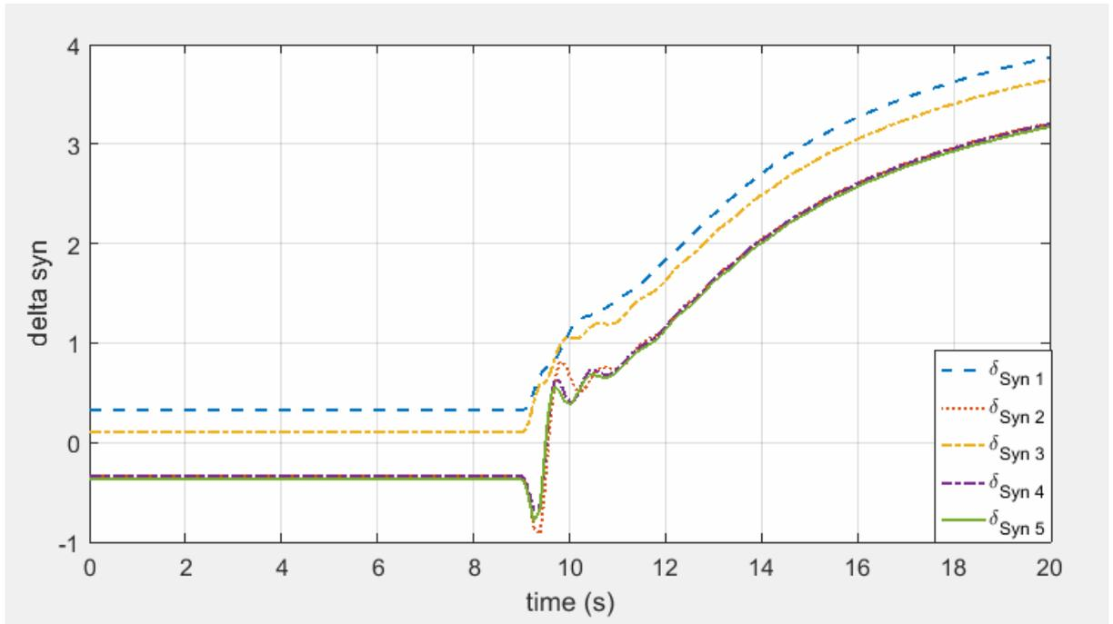
**Fig. 16. Represent delta against Time for All Generators When the Fault Occurs At Bus No.2 – Without Control**
