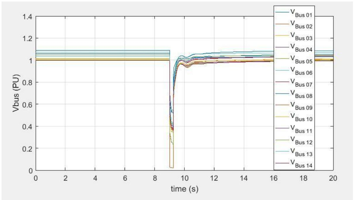
fig.20. Represent Voltage against Time For All buses When The Fault Occurs At Bus No.2 – With AVR, TG and PSS Control
