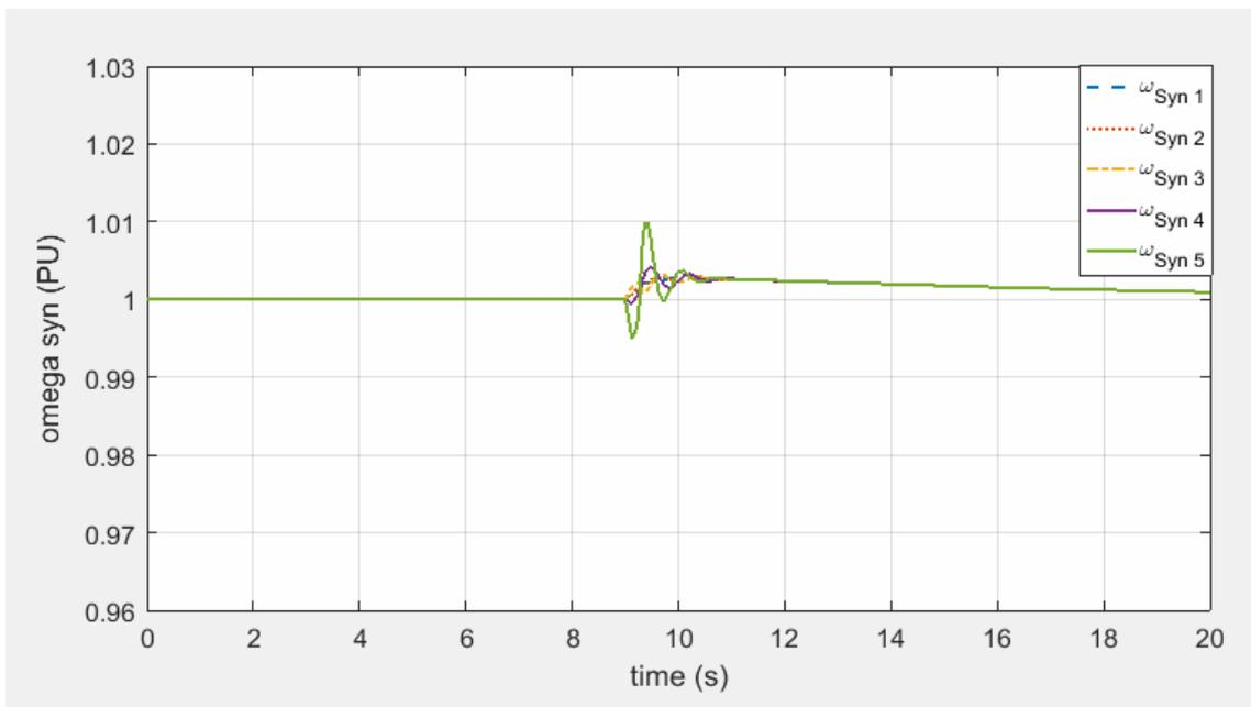
**Fig. 13. Represent Speed against Time for All Generators When the Fault Occurs At Bus No.11 – Without Control**
