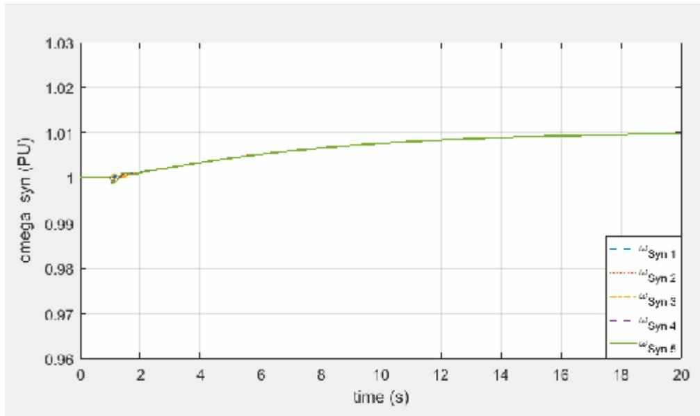
**Fig.22. Represent speed against Time for All Generators When the line 2-4 outage from the network without control**
