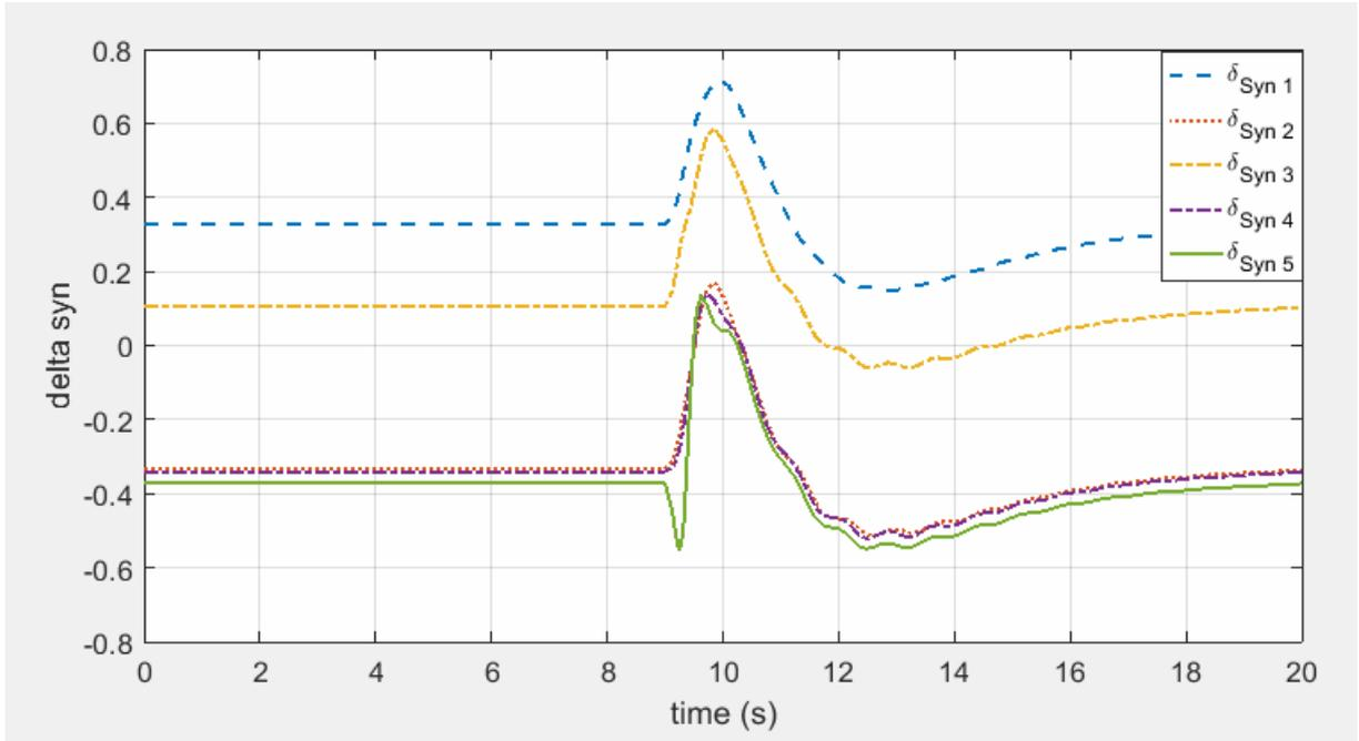
**Fig. 12. Represent Delta against Time for All Generators When the Fault Occurs at Bus No.11 - without Control.**
