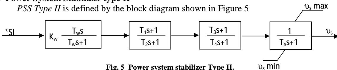
Fig. 5 Power system stabilizer Type II.
