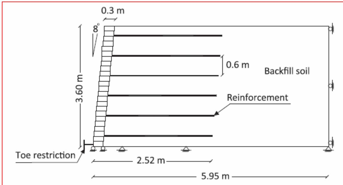
Fig. 1 Schematic section of wall W1 (Hatami and Bathurst 2005).
