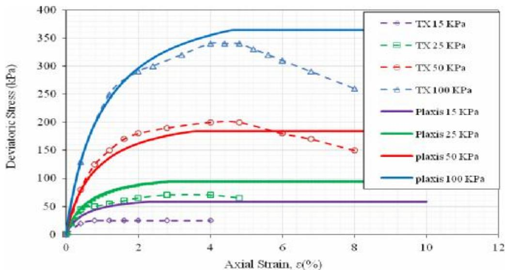
**Fig. 5 Stress-strain response of RMC sand for tri-axial sample tests (Lee, 2000) versus developed Plaxis 3D model simulation**
