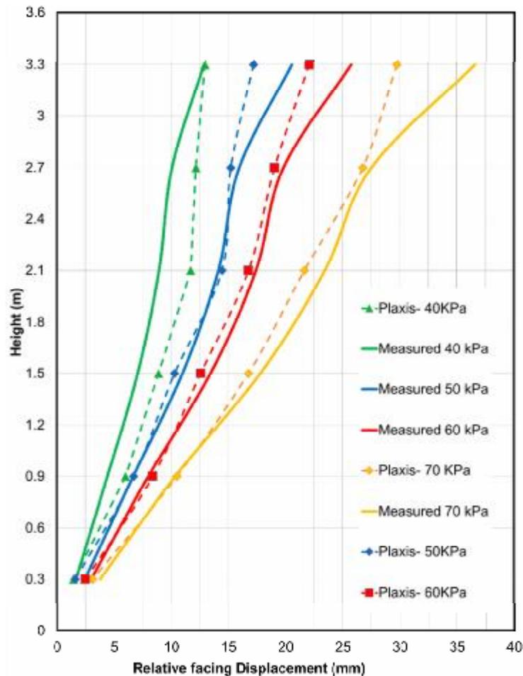
Fig. 8 Relative facing displacement at EOL; Plaxis results versus monitoring records
