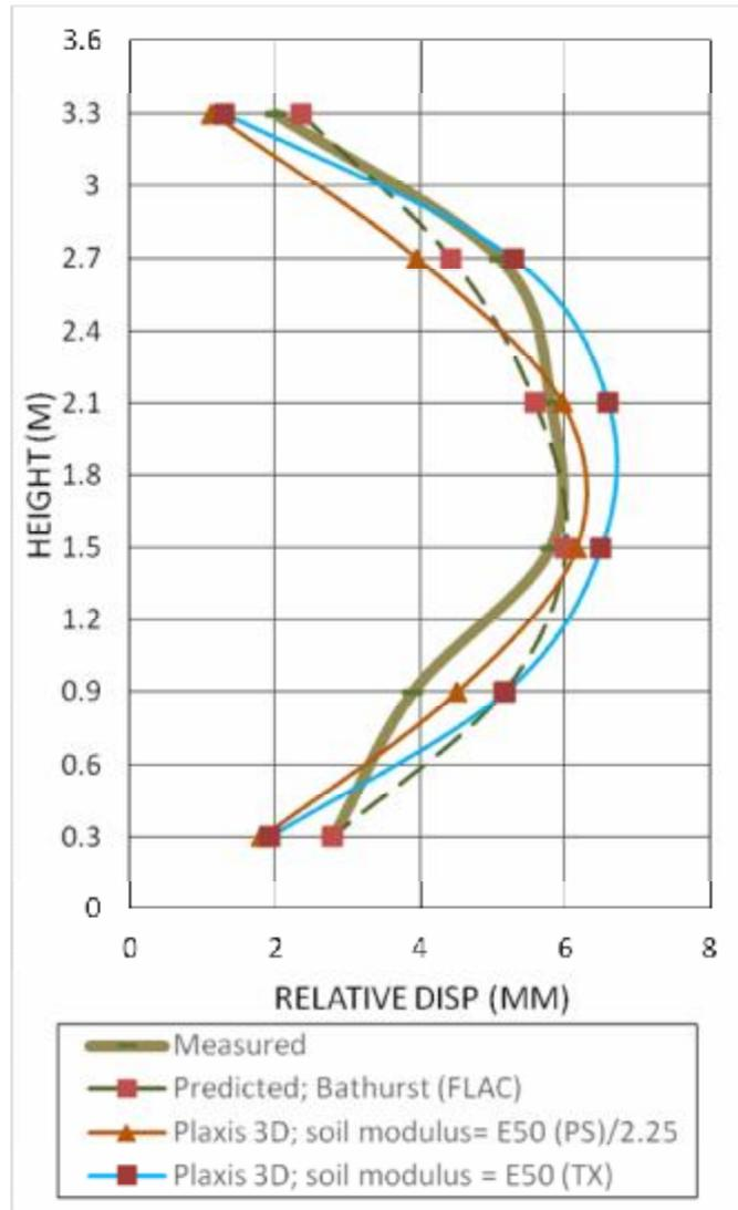
Fig. 7 Relative facing displacement at EOC, validation model trails
