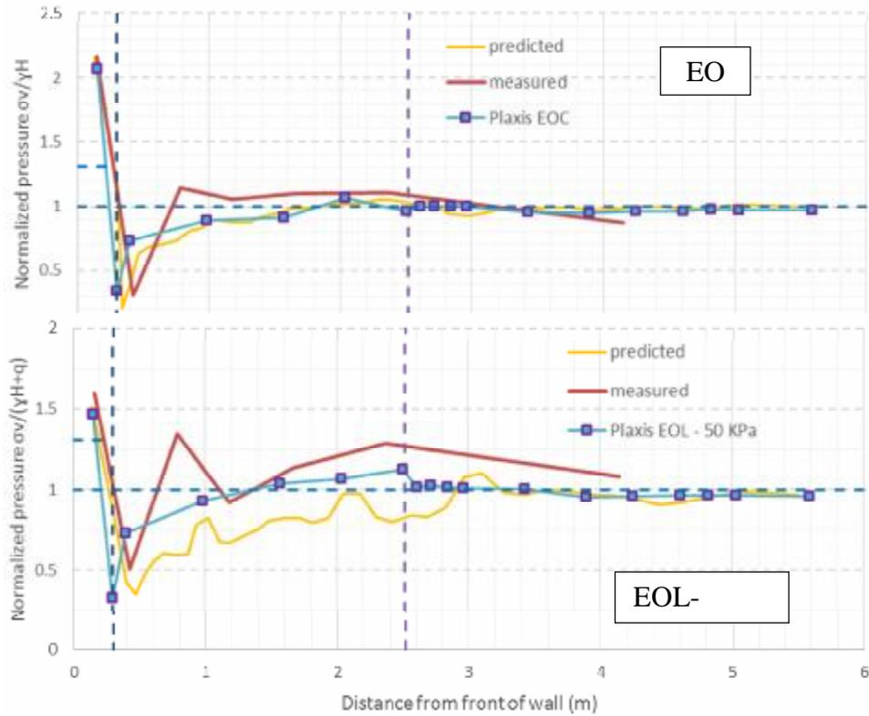
Fig. 11 Foundation vertical stresses at EOC and EOL- 50KPa; Plaxis results versus monitoring records
