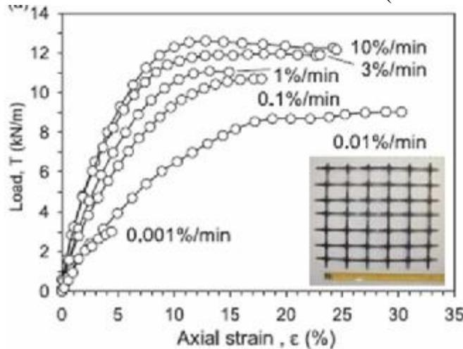
**Fig. 2 In-isolation Load- Strain response of Polypropylene geogrid specimens from Constant Rate of Strain (CRS) tests results (Hatami and Bathurst 2005).**
