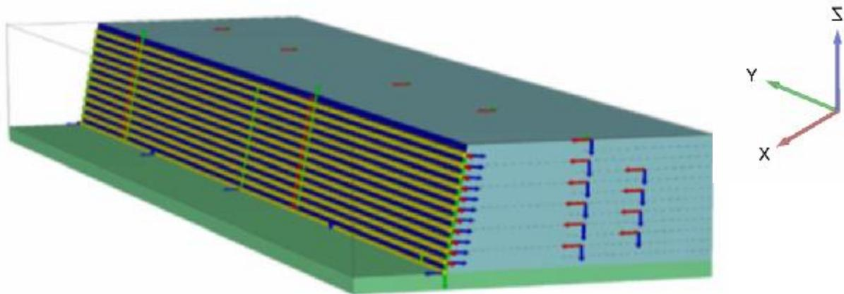
Fig. 4 Configuration of Plaxis 3D model validation for RMC wall (W1).
