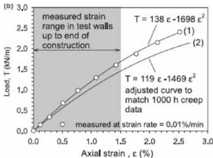
**Fig. 3 In-isolation Load- Strain response of Polypropylene geogrid specimens from Constant Rate of Strain (CRS) tests results (Hatami and Bathurst 2005).**
