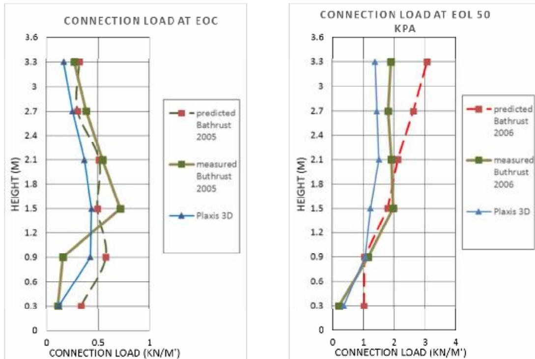
**Fig. 10 Connection loads for EOC and EOL- 50KPa; Plaxis results versus monitoring records**
