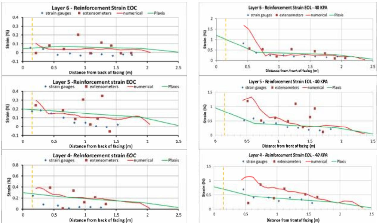
Fig. 12 Geogrid strain at EOC and EOL- 50KPa; Plaxis results versus monitoring records
